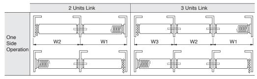
For right operation, install the brackets on the left side as the part shown at right.
